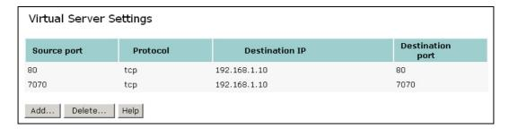
The WEBcam can always dynamically obtain an IP address instead of a fixed one. However, since there is a direct link between a port and a specific IP address in the virtual router, the service only functions while the WEBcam has no other address. In this case, it is recommendable to assign the MAC address of the WEBcam permanently to an IP address → see DHCP / Address Reservation.
